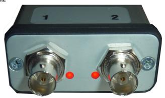
800 MHz with a stability of better than 1e-9 (1 part per billion (ppb) within 1 minute after achieving lock to the high accuracy GPS Satellite Network which is controlled by a Caesium Clock with accuracy approaching 1e-12
